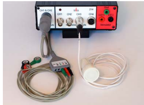
Figure HH-2-3: The ECG cable and event marker connected to an IWX/214.
