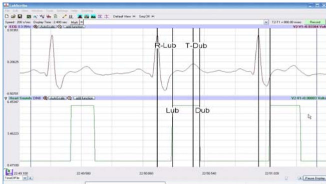
Figure HH-2-6: ECG and event marker recordings displayed in the Analysis window. Lines and labels were added to the figure to indicate the locations where cursors should be placed to measure the time intervals between the R wave and the "lub" and the T wave and the "dub".
