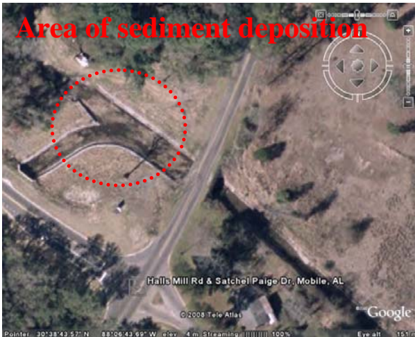
Figure 2: Google Earth image of sediment deposit in Bolton Branch at Halls Mill Road circled in red.
